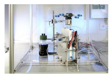
Figure 1: Vanadium/Oxygen cell based on two membranes
