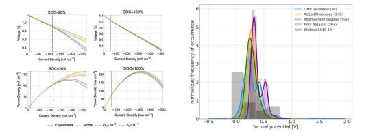
Figure 1: left) Simulated vs. experimental polarisation curves based on a OD cell modell for MV/TMA-TEMPO, right) MLbased calculated formal potentials vs. database-based potentials of a dataset with 9000 quinone based redox couples
