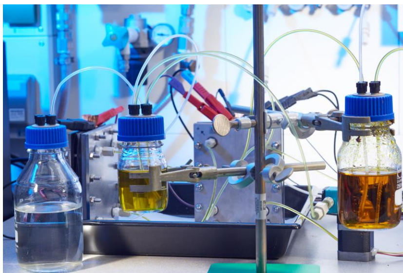
Figure 1: Picture of a laboratory scale Iron/Iron redox flow battery with recombination cell
